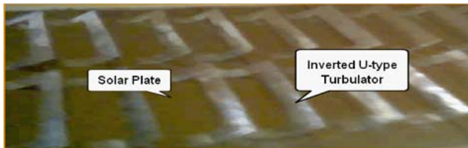
Fig. 2: Photograph of turbulator roughened absorber plate
