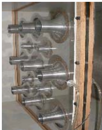
Fig. - 6: Photograph showing the back view of the set of nozzles in the test bed
