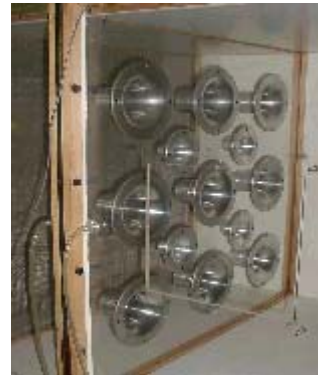
Fig. - 5: Photograph showing the front view of the set of nozzles in the test bed
