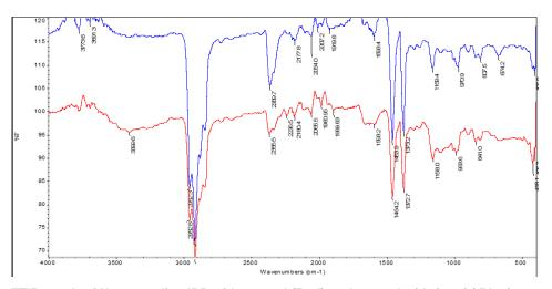
Fig. 1: FTIR result of Non-metalizedPP with control (Red) and treated with fungi (Blue) spectrum.
