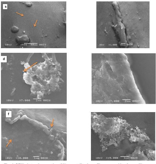
Fig. 4: SEM photomicrographs of Non-metalized cpp film exposed by *Aspergillus spp* and *Pencilliumsppat* (a)500x (b)1000X (c)7000x (d)10,000x (e)15000x respectively after 30 days of incubation
