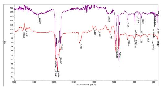
Fig. 2: FTIR analysis result of metalized (red spectrum control) and metallized film (purple spectrum) after treated with fungi.
