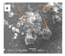
Fig 3: SEM photomicrographs of metalized cpp film exposed by *Aspergillus spp* and *Pencilliumsppat* (a)500x (b)1000X (c)7000x (d)10,000x (e)15000x respectively after 30 days of incubation
