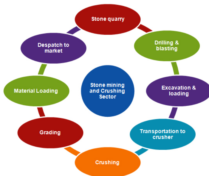
Fig. 1: Material and activity flow of stone quarry and crusher operation
