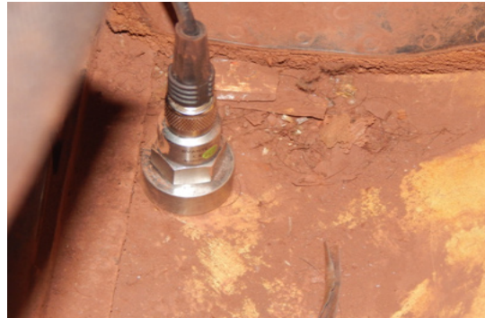
Fig. 3: SV80 mono-axial accelerometer magnetically secured to the floor of the driver's cabin
