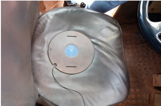
Fig. 2: A tri-axial seat-pad accelerometer placed on the seat of the operator
