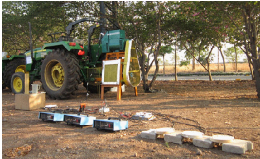
Fig. 4: PTO driven generator with AC load
