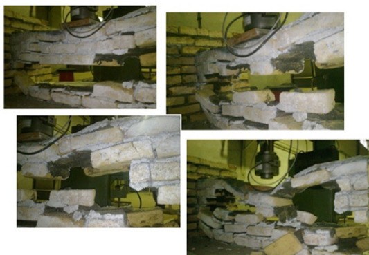
Fig. 8: The diagonal cracking development until the complete failure of non-reinforced beam
