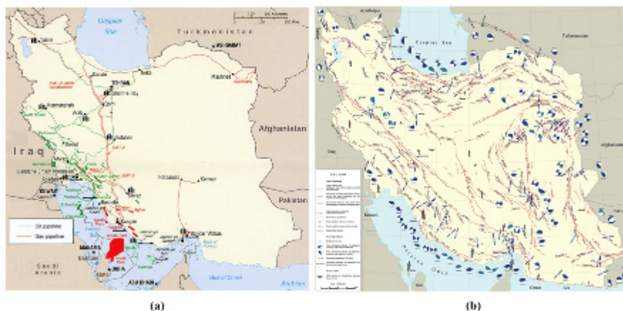
Fig. 2: (a) national oil and gas pipeline network of Iran, (b) potential fault map of Iran
