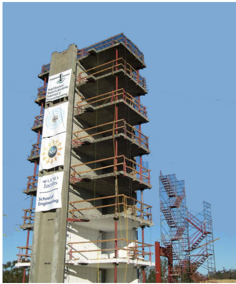
Fig. 3: Seven-storey Concrete Building with Shear Wall
