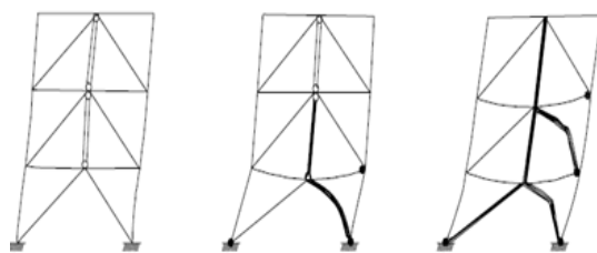
Fig. 2: Partial-height zipper mechanism (Yang , 2006)
