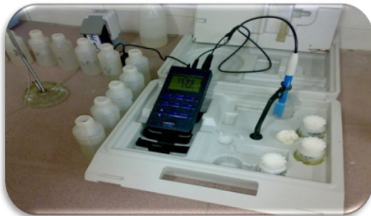
Fig. 8: PH measurement by a digital pH meter.
