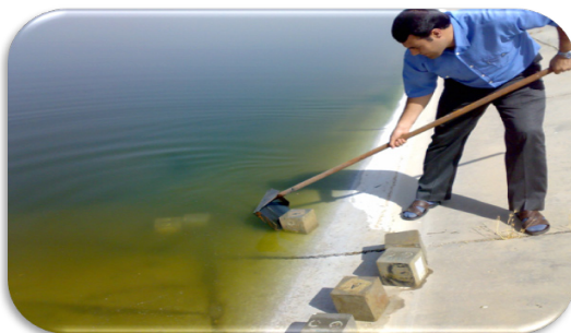
Fig. 6: Arrangement of samples in basins.
