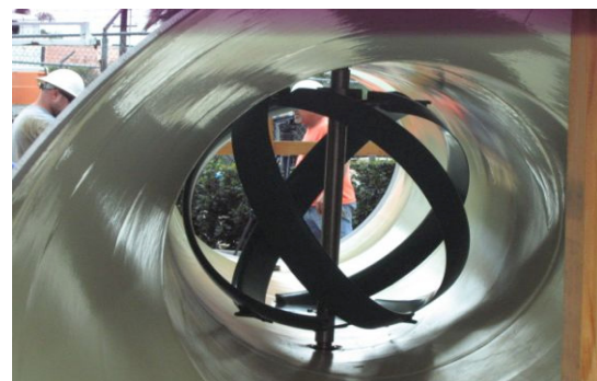
Fig. 2: Single spherical turbine installed inside a pipe 8
